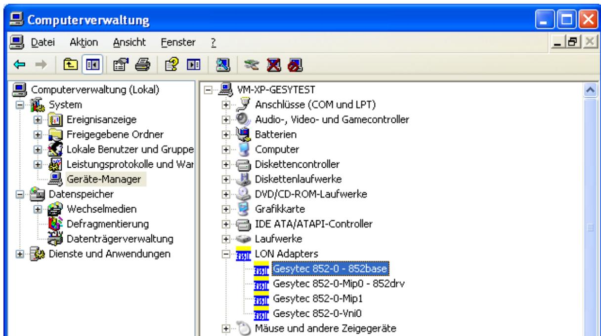
Editing the driver properties allows modifying the driver names. MIP drivers can be used by applications which are not LNS based, e.g. the Easylon OPC Server M, or Echelon’s nodeutil or NLUTIL. Honeywell’s Excelon is as well running
