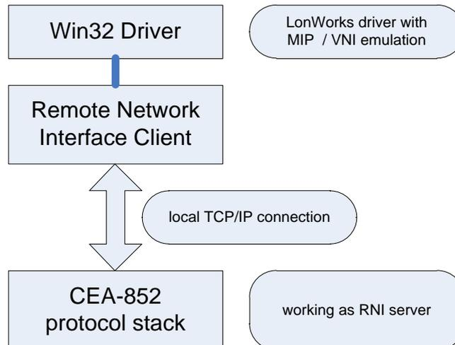
Both applications, the CEA-852 protocol stack and the remote network interface client will run as a service, to ensure that any software, which is running as a service as well, can use Lon over IP without user log in.
