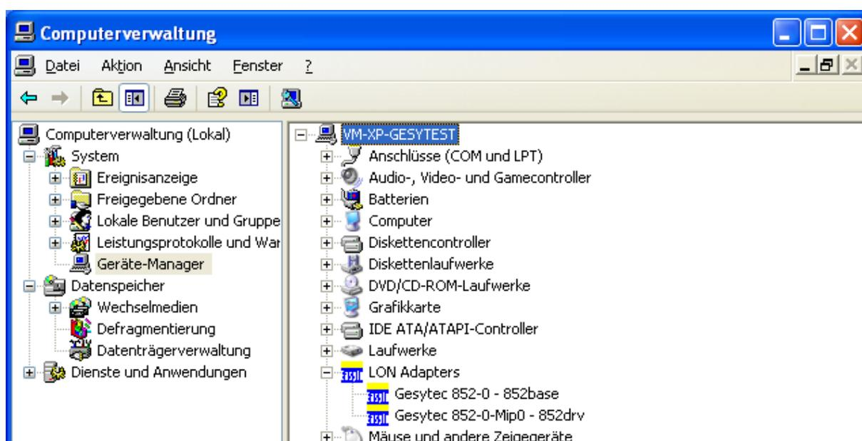
Accessing the properties of the 852base in the device manager allows to individually configuring its settings. We recommend installing 2 MIP and 1 further VNI instances. For this purpose double-click the "Gesytec 852-0 852base" entry, go to the extended properties and enter "2" for the "Number of MIP-Interface" and "1" for the "Number of VNI-Interfaces". "OK" will set these values and drivers will be installed accordingly.
