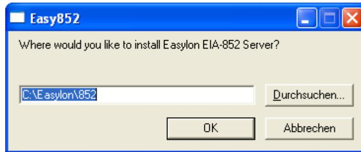
Now the setup installs the whole software. The setup finishes with the prompt for the parameters of the CEA-852 protocol stack. All settings can later be modified via the Windows Start menu: “**Programs->Easyton->852->Config 852 Interface**”.
