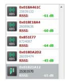
The Inputs section shows the EnOcean devices that will be converted into BACnet data points. To generate data points the gateway needs to know the sensor's EEP as this defines what data point will be created. Therefore only EnOcean sensors which have been recognized can be assigned. Sensors with icons indicate the type of message only (i.e. 4BS, VLD, MSC) cannot be assigned and will be highlighted in red to indicate the problem.
